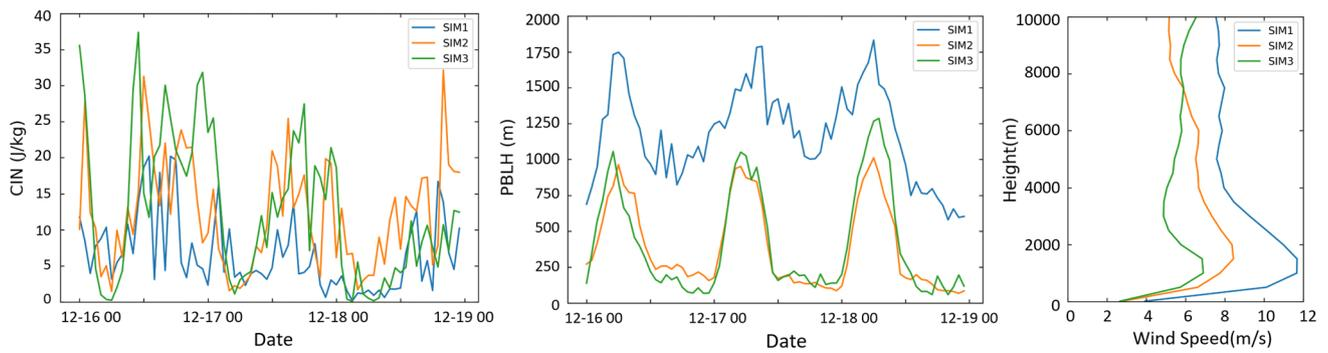
**Fig. 11** Time series of station averaged CIN (left) and PBLH (middle) corresponding to different PBL schemes. Station averaged wind speed (right) at different level averaged for the period from 0000 UCT 16<sup>th</sup> December 2021 to 2300 UCT 18<sup>th</sup> December 2021
